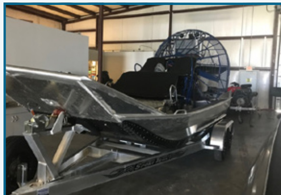
At 17 feet long, the airboat has a cruising speed of 40 mph and seats a driver plus four people.
