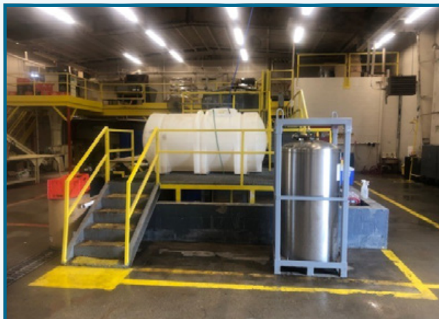
The mixing of the hand sanitizer occurs in a 700-gallon poly tank at Prison Enterprises.
