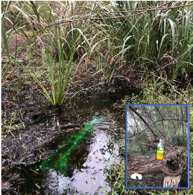
Figure 5 – Visualization of flow in the effluent application zone (Zone 1) using fluorescent dye.
