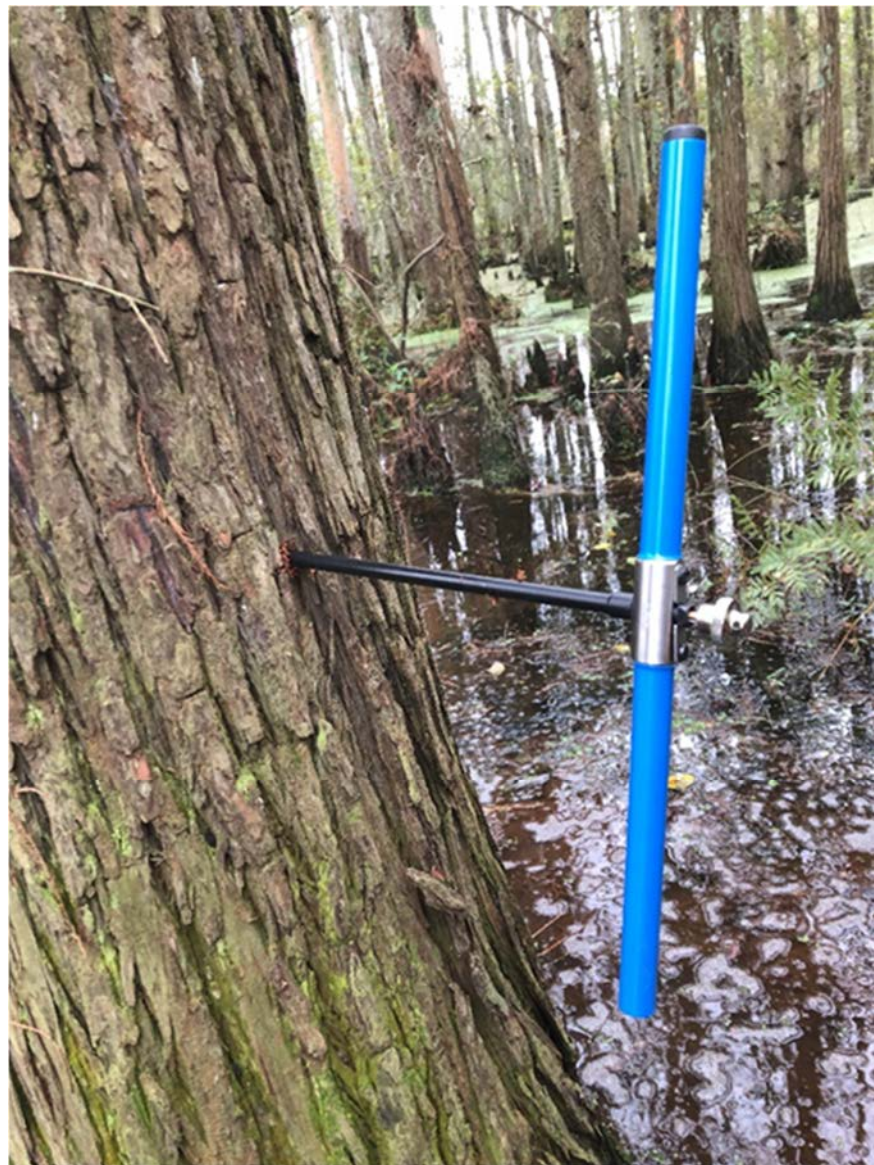
Figure 8.1 – Use of increment borer at the Hammond MID location, November 14, 2018
