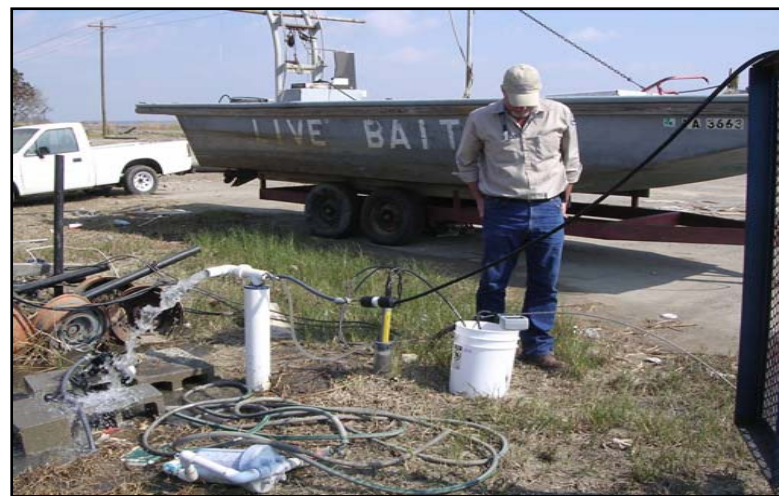
Geologist John Jennings samples a well in St. Tammany Parish. He uses a YSI field meter to check the pH, conductivity, salinity and temperature of the water.
