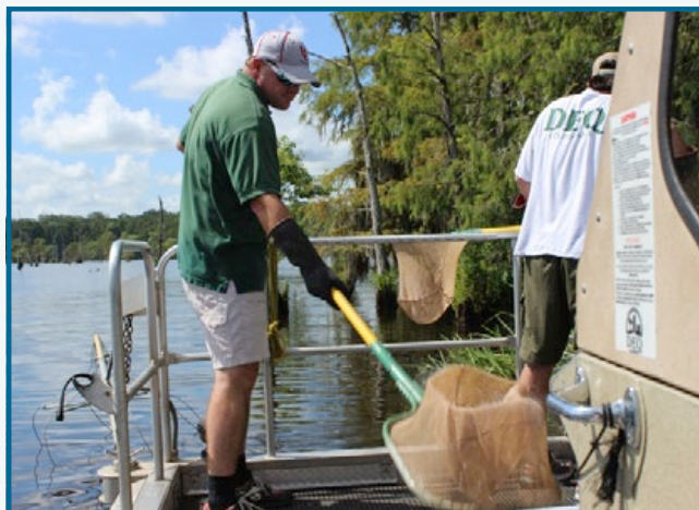
LDEQ Environmental Scientist Staff Shane Miller (left) transfers sampled fish from a scoop net into a holding tank. The tentacle-like electrode apparatus (lower left) temporarily stuns nearby fish, which makes it easier for the team to select and retrieve a variety of species.
