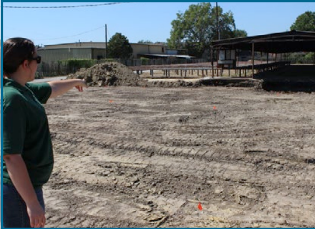
Environmental Scientist Jane Hebert from DEQ's Acadiana Regional Office identifies orange flags that denote soil sampling spots at the remediation site.
