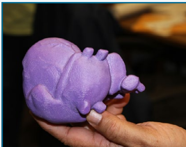
LSU researcher Michael David Vincent holds a form for a human heart. The form was made on a 3D-printer of plastic produced from byproducts of the energycane/sorghum to butanol process at the Audubon Sugar Institute. The plastic is biodegradable, and once it is seeded with stem cells, tissue grows around the form. The form then degrades and disappears, leaving a human heart.
