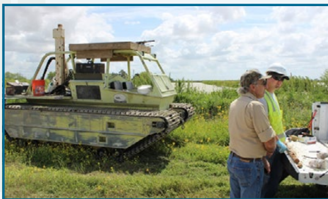
A track-mounted boring device collects samples next to a crawfish retention pond in Acadia Parish as DEQ Environmental Scientist Terry Sylvester, left, confers with a contractor
