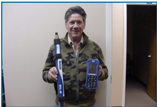
DEQ Environmental Scientist Jeff Dauzat displays the new Hydrolab HL4 sonde and the surveyor HL, which reads the data from the sonde.
