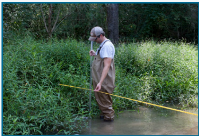
DEQ Environmental Scientist Zach Herrington conducts a wading flow measurement at Big Creek in Tangipahoa Parish.
