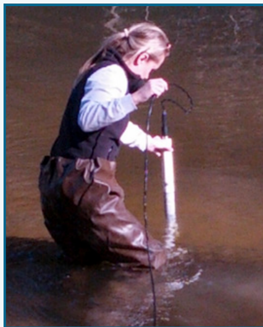
DEQ Environmental Scientist Davina Witte lowers a Hydrolab MS5 sonde into the Tchefuncte River for an insitu water analysis.
