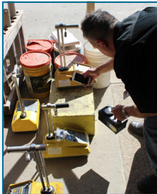
Russell Clark conducts a device inventory and also performs radiation surveys of several Troxler 3440 soil moisture density gauges at a soil testing engineering firm in Baton Rouge.
