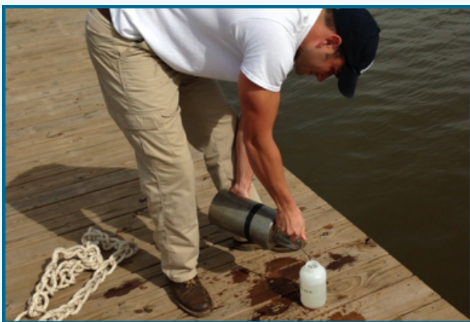
After the water sampling canister is filled, the sample is poured into various containers for subsequent testing in a lab
