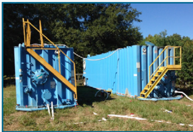
Two 21,000-gallon Baker Tanks process groundwater at Geosyntec's biobarrier site number 1 in Monroe.
