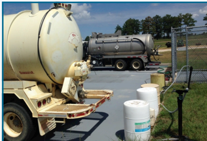
Gray water collected in the field during training exercises is transported and processed at a wastewater treatment site at the Recycling Center.
