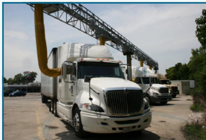
*Trucks using IdleAir connections at Cash's Truck Stop at Interstate 10 exit 151 in Port Allen*
