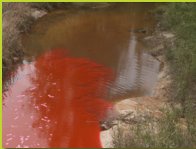
Red dye in stream used for water survey
