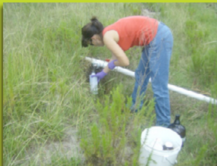
Sampling an "air-lift" well that supplies a stock pond.
