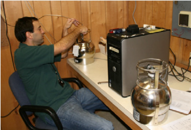
DEQ Environmental Scientist Cory Parent checks an air monitoring canister, which collects an array of airborne compounds for further lab analysis
