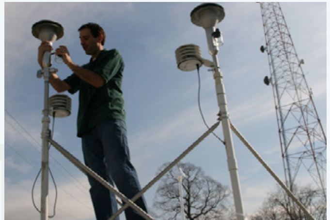
DEQ Environmental Scientist Cory Parent checks a Beta Attenuation Monitor (BAM) atop the Capitol Air Monitoring Station in Baton Rouge
