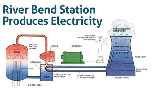
A nuclear power plant uses steam to generate electricity. Steam, created by heating water through energy produced by a nuclear reaction, drives turbine blades to spin. This rotational energy is then converted to electrical energy by a generator.
