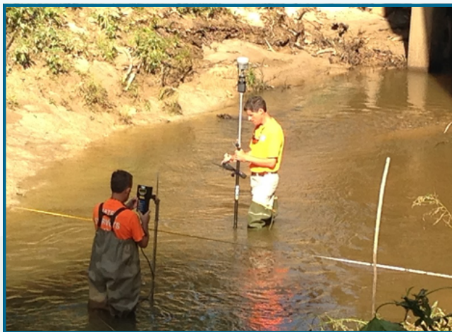
LDEQ Environmental Scientists Chad Keith (l) and Eric Garner measure the flow rate and verify the GPS location information at a water sampling point in a waterway in Tangipahoa Parish.
