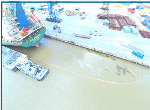
Absorbent boom was placed around the spill for containment purposes.
