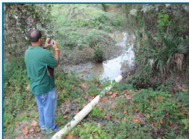
Sean Darensbourg observes the outfall from a discharge pipe adjacent to the wastewater treatment plant. Obstructions in the pipe, proper flow, color and consistency of the receiving stream and the presence of any odors will be noted in the Field Interview Form.
