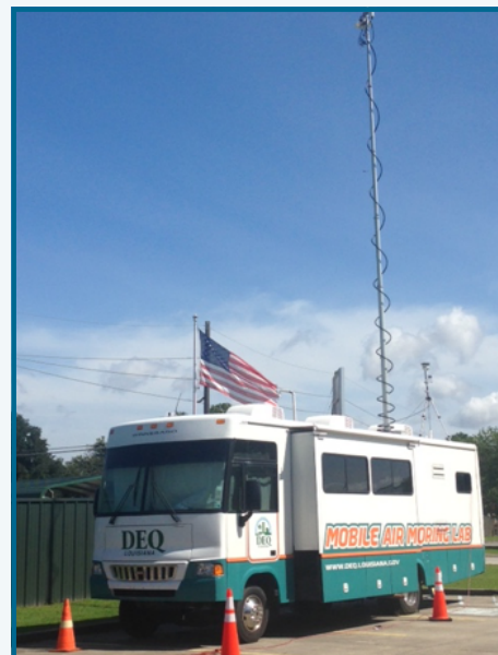
The MAML can be deployed across the state to conduct air monitoring for a wide array of constituents.
