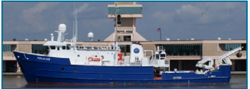
The Pelican – LUMCON's Oceanographic Research Vessel. The main deck runs the length of the vessel and covers approximately 1,056 square feet of open aft deck and about 1000 square feet of interior deck space forward. The ship's 3 main labs: bottle lab, wet lab, and dry lab are located on the main deck, along with the galley and mess areas, electronics lab, and cold non-scientific cold storage facilities.
