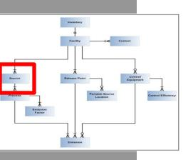
Source – Equipment or unit that generates emissions. This is the operating equipment, not the control equipment or the stack/vent
