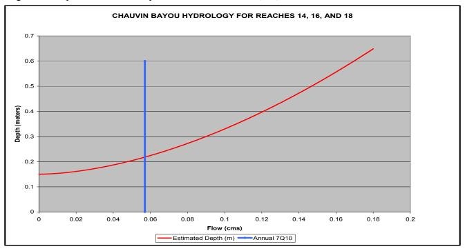
Figure 3 - Depth vs Flow for Bayou Chauvin Reaches 14, 16, and 18
