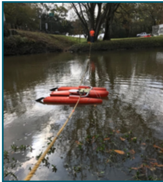
Figure 3. Jacie Ourso and Chad Keith taking flow measurements from the banks of ambient site, 0676 [Bayou du Portage at Parish Rd 679], with the RiverPro 1200 purchased with 319(h) funds.
