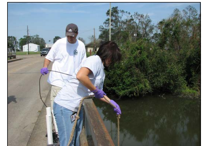
Geologists Jesse Means and Tiffani Cravens perform surface water sampling on Bayou Lafourche following Hurricane Gustav in order to assess impacts of the storm on the bayou, a drinking water source.
