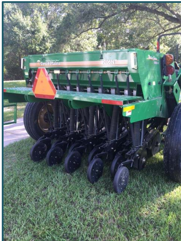
Figure 3 Seven foot No-till grain drill located at the Bayou Vermillion District, Lafayette, LA
