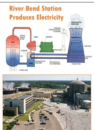
A Nuclear power plant uses steam to generate electricity. Steam, created by heating water though energy produced by a nuclear reaction, drive turbine blades to spin. This rotational energy is then converted to electrical energy by a generator.
