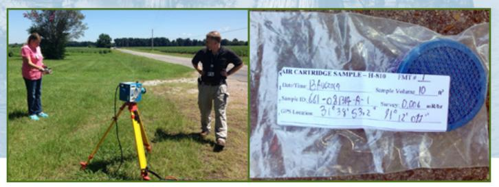
LEFT: DEQ Environmental Scientist Carolyn Bourn (left) takes air samples from a handheld survey meter in Tensas Parish as Environmental Scientist Michael McMahon, serving as field team controller for the drill, checks the mounted air volume totalizer. RIGHT: Air samples are stored in cartridges and filters which are then sealed and labeled for submission to a laboratory.
