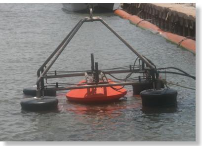
There are a variety of skimmers that can be deployed during the oil cleanup phase.
