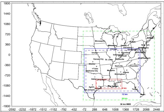
**Figure 4-1a.** Nested 36/12/4 km modeling domains for the Baton Rouge 8-hour ozone modeling study. Dotted line domains are for CAMx/EPS that are nested in the MM5 solid line domains.
