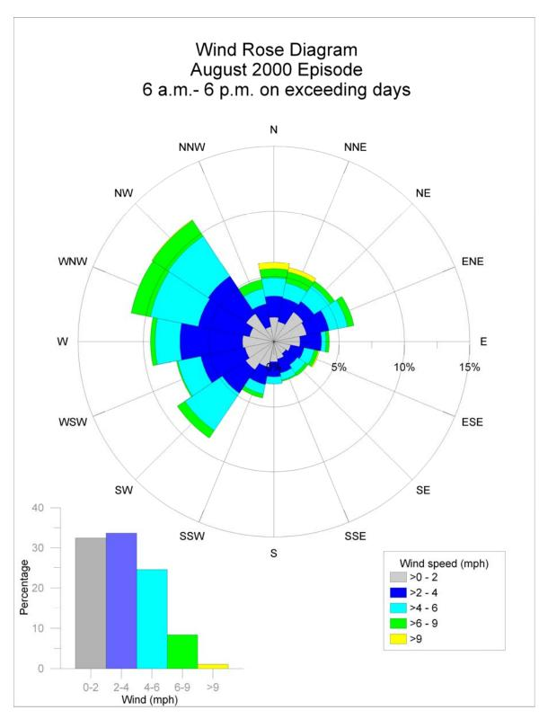
**Figure 3-22.** Wind rose based on hourly wind speed/direction data from all Baton Rouge monitors between 6 AM and 6 PM on exceedance days.
