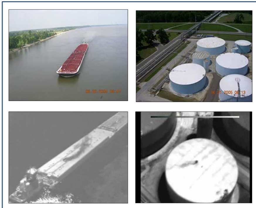
Figure 3.1-1. VOC leak detection with the HAWK IR camera system.
