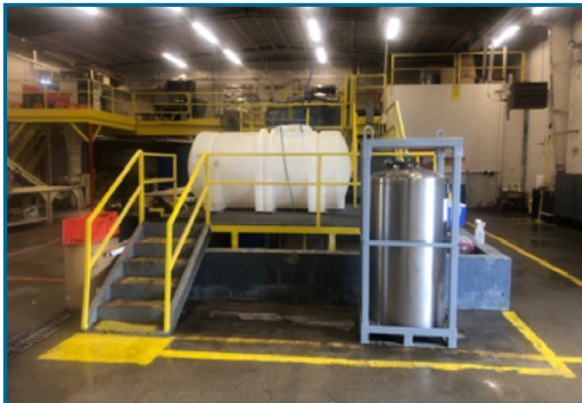
The mixing of the hand sanitizer occurs in a 700-gallon poly tank at Prison Enterprises.
