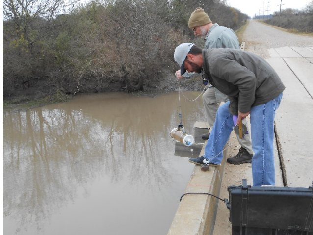
Figure 4 UL employees using a Van Dorn sampler for water quality sampling in Bayou Chene
