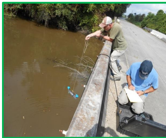
Figure 2 Water Quality Sampling Using a Van Dorn Sampler, and Determining Field Parameters Using an YSI Sonde
